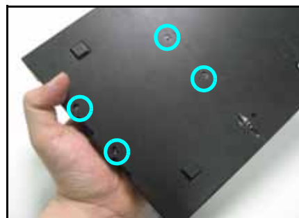
Figure 27.2 Support the HDD with your hand and remove mounting screws.
